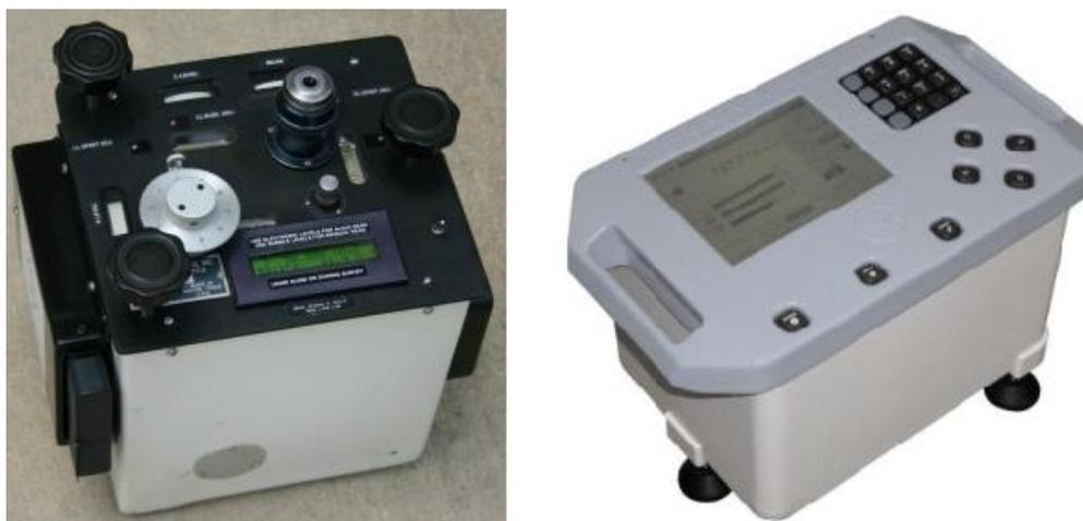
Fig. 5-9 Show two models of LaCoste-Romberg gravimeters. Aliod G gravimeter (left side) and EG gravimeter (right side).
