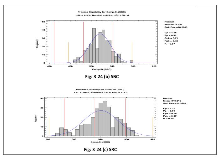
Figure (3-24): Process capability for Comp.st. (OPC, SBC and SRC)
