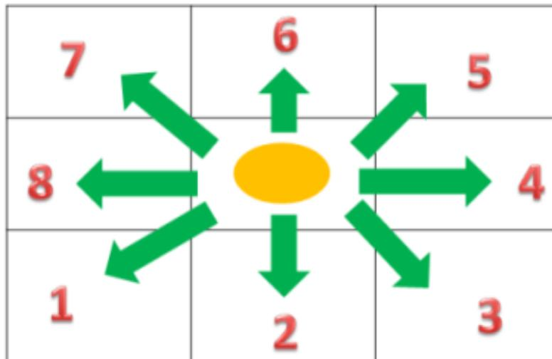
Figure 3. 8 Illustrates the directions of the agent's movement
