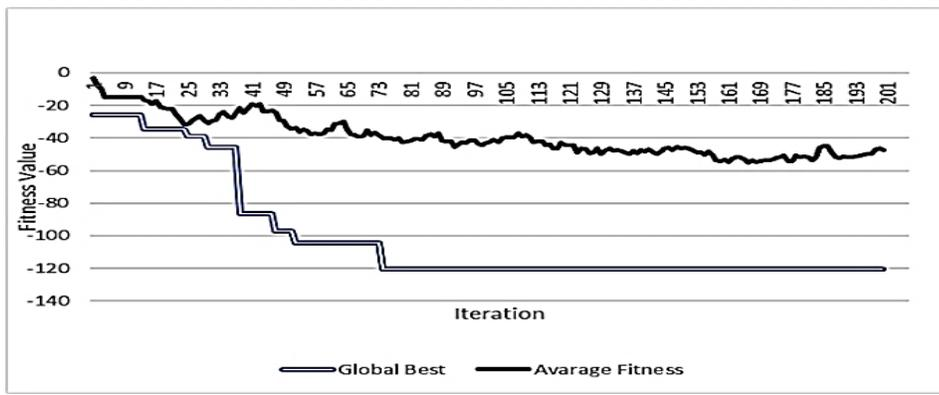
Figure 4. 9 Presents average fitness and global best as a result of optimizing aperiodic antenna array designs in 200 Iteration with 20 artificial scout bees using standard FDO
