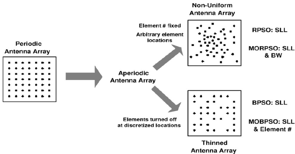
Figure 4. 7 Presents a thinned antenna array and Non-Uniform antenna array
