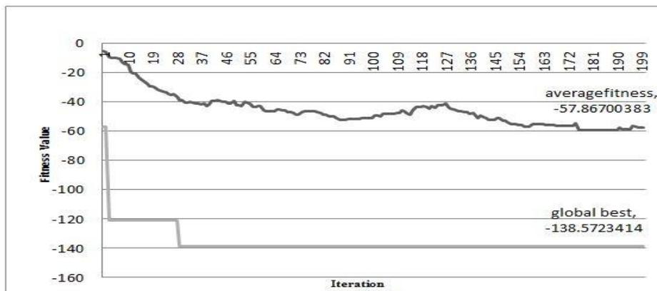
Figure 4. 10 Presents average fitness and global best as a result of optimizing aperiodic antenna array designs in 200 Iterations with 20 artificial scout bees using IFDO
