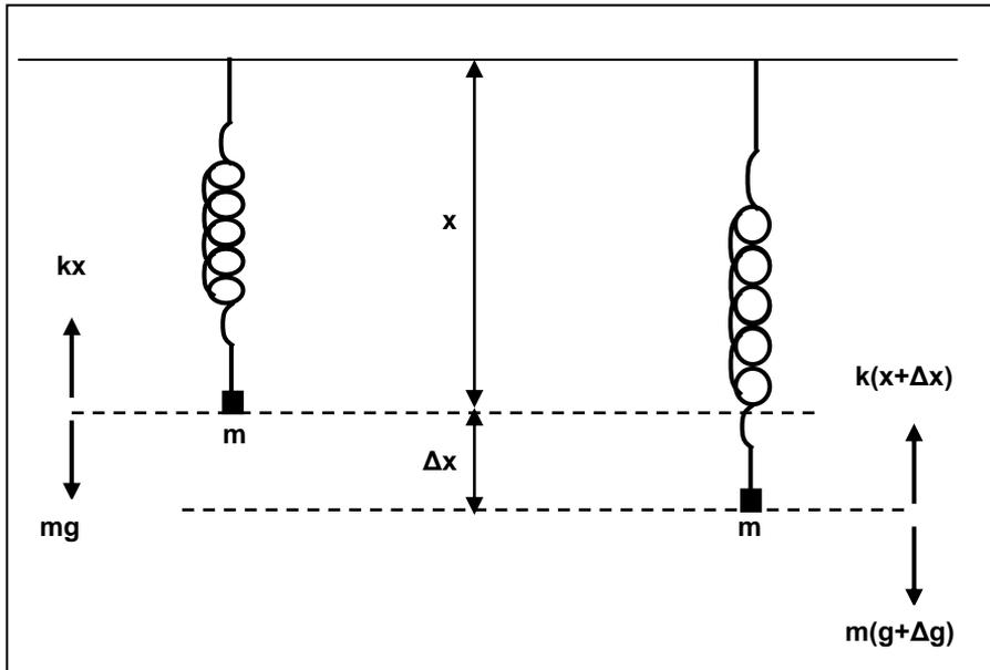
Fig. 5-4 Principles of the spring balance
