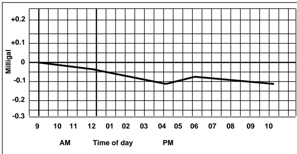
Fig. 5-10 Example of a drift curve
