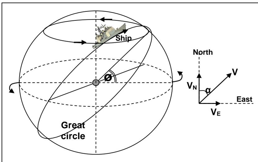
Fig. 6-7 Generation of an additional centrifugal acceleration due to the motion of the gravimeter-carrying ship over a segment of a great circle and at the same time rotating about the Earth polar axis .
