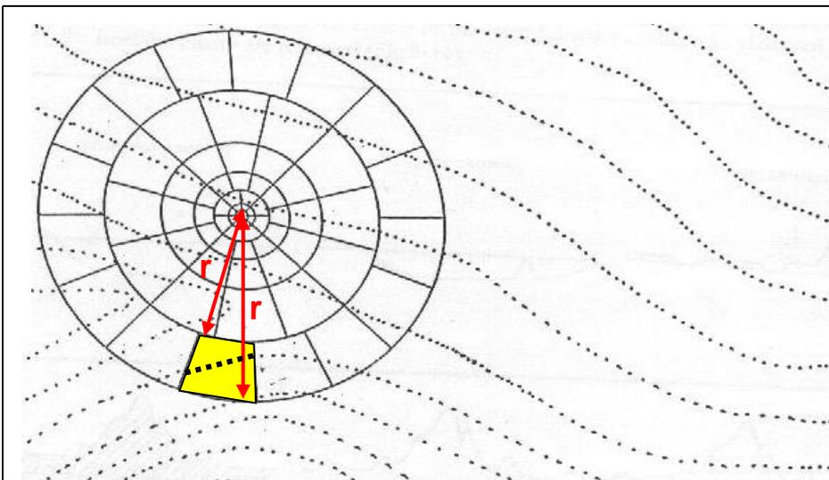
Fig. 7-11 The procedure followed in calculating terrain correction by use of the Hammer chart. Average elevation of the yellow compartment is estimated from the contours crossing it.
