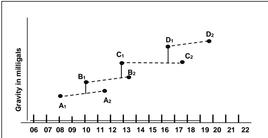
Fig. 6-2 Base station re-occupation technique for determining the short term tide-drift curves which are used to establish the base-station network.
