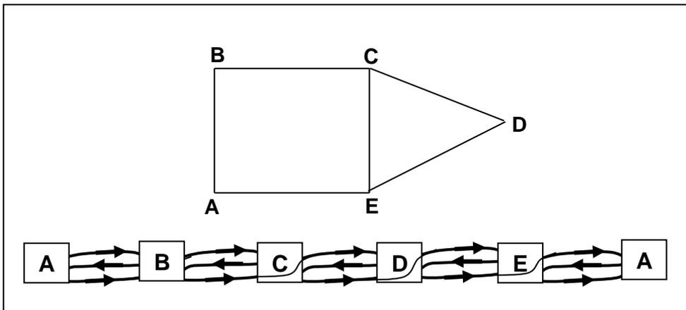
Fig. 6-3 Looping-method applied in the process of establishing a base-network made-up of five base stations ( A, B, C, D, & E )
