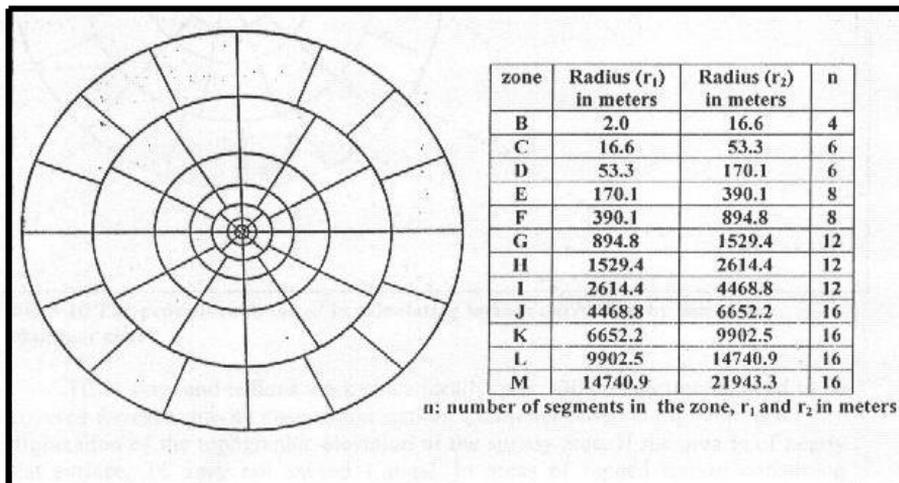
Fig. 7-10 Part of the Hammer chart. The complete chart consists of zones (B, C, D, ..., M) varying in radius from 2m for zone-B to 22km for zone-M (Kearey and Brooks, 1987, pp 152-153)
