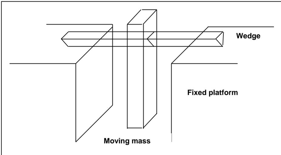
Fig. 5-3 Sketch showing the structure of the Gulf pendulum.
