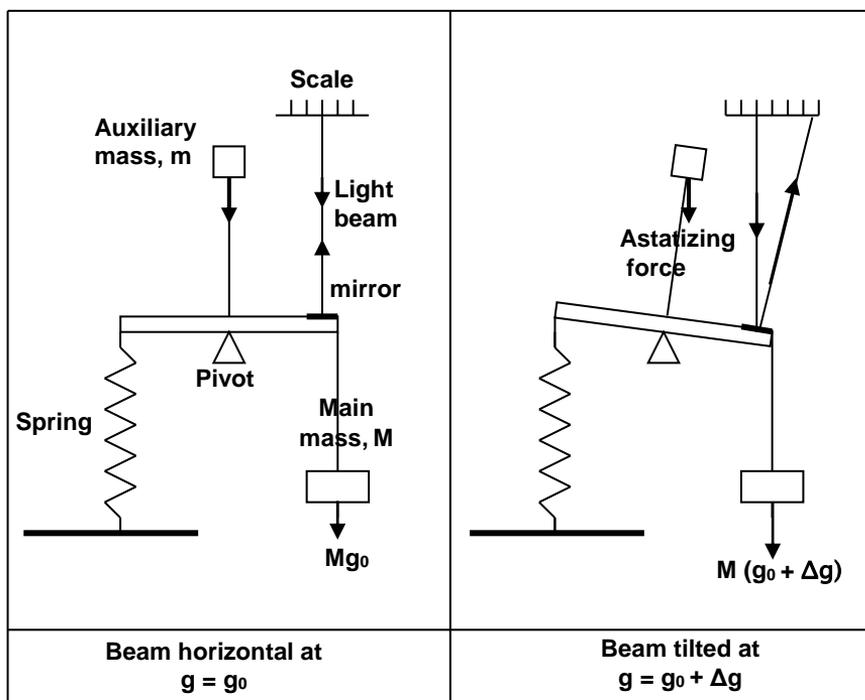
Fig. 5-7 Schematic representation of the Thyssen gravimeter.
