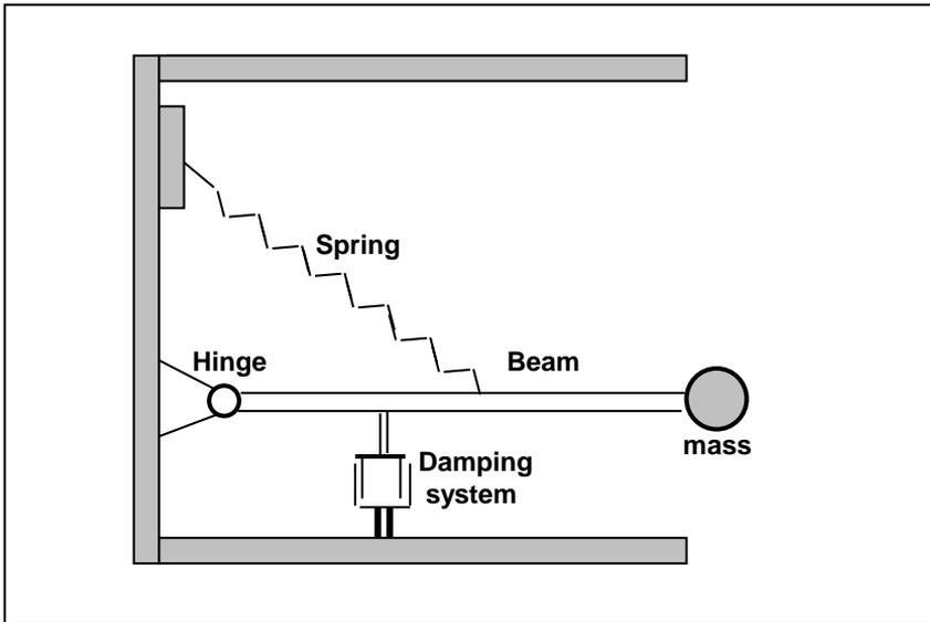
Fig. 6-6 Principle of beam-damping system fitted to shipboard gravimeter.
