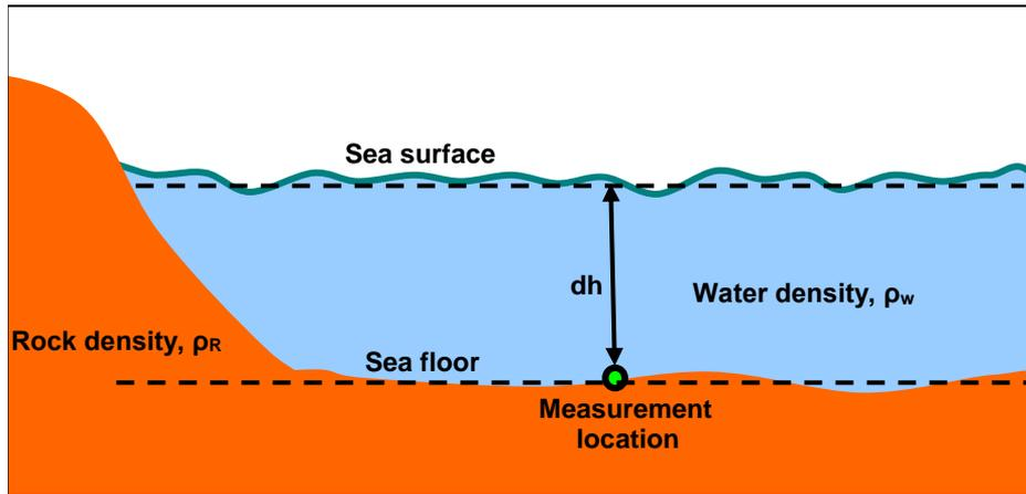
Fig. 7-13 Bouguer correction for the case of sea-floor gravity measurements
