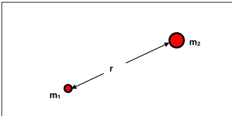
Fig. 2-1 Attraction force ( $\mathbf{F}$ ) between two masses;  $\mathbf{m}_1$  and  $\mathbf{m}_2$  at distance  $\mathbf{r}$  apart.
