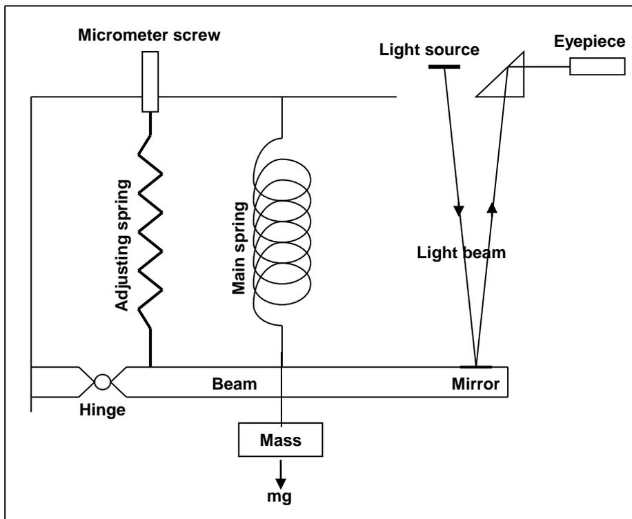
Fig. 5-5 Schematic representation of the Hartley gravimeter
