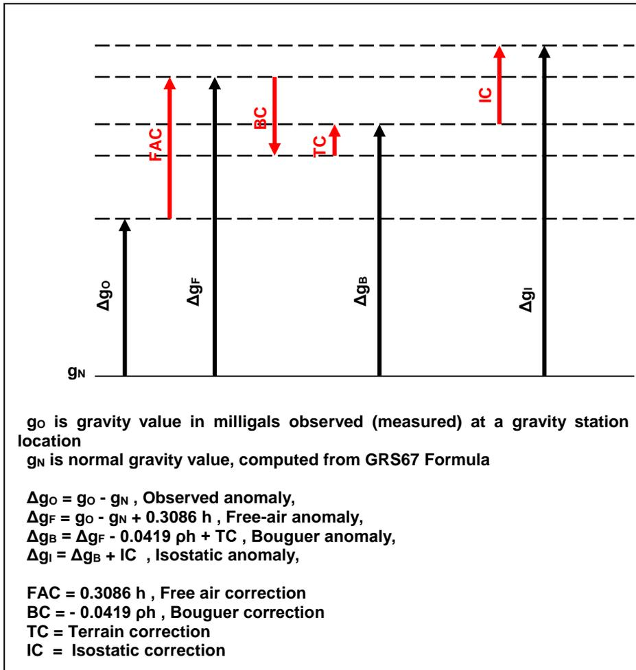
Fig. 7-12 The processing sequence normally followed in gravity data-reduction.
