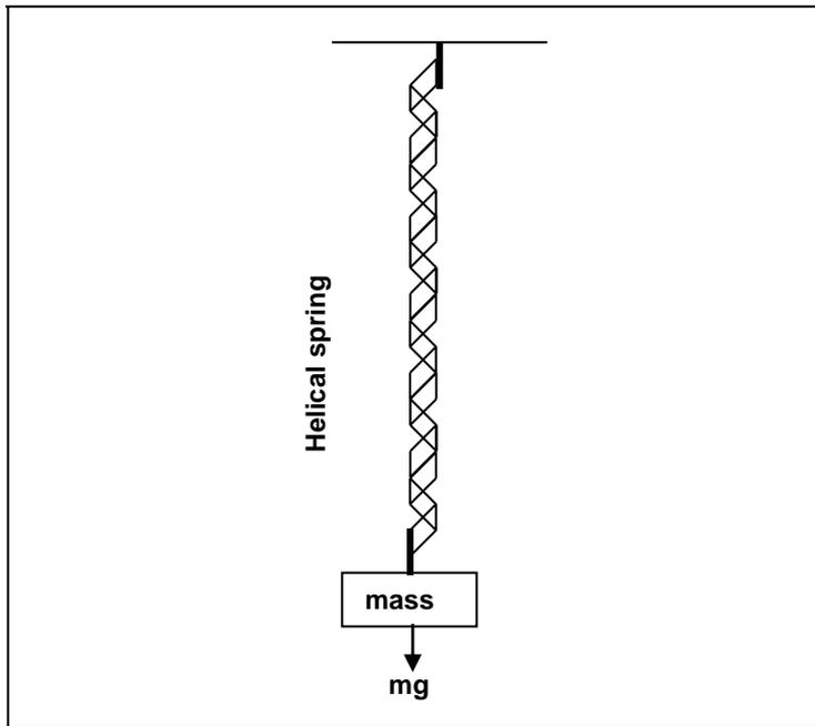
Fig. 5-6 Schematic representation of the Gulf gravimeter.
