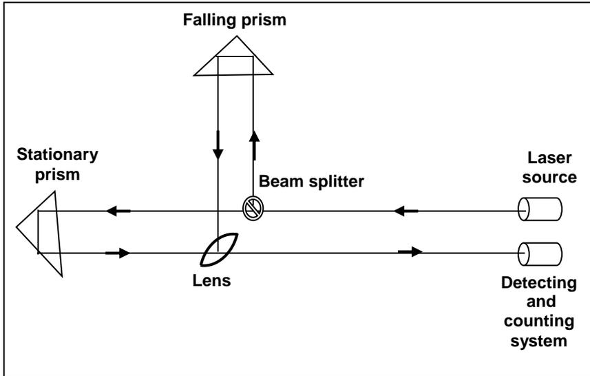
Fig. 5-1 Sketch layout of the falling-prism instrument for measuring gravity
