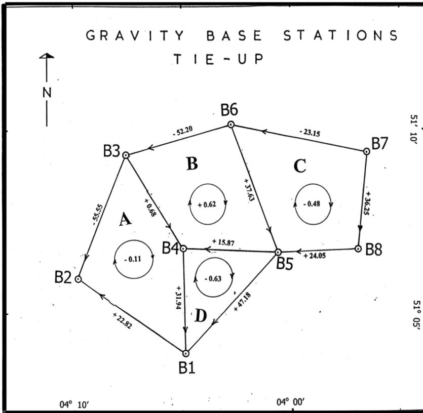
Fig. 12-3 Base-station network (forming four compartments) with the computed closing-error values (a, b, c, d). Arrow direction indicates relative increase in gravity value between base stations.
