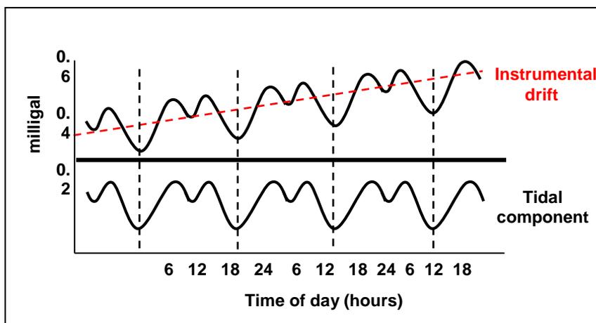
Fig. 4-5 Time-variant gravity variation. The cyclic (tidal) component superimposed on the none-cyclic instrumental drift (the dotted line). The lower curve represents the time-variant gravity variation (tidal component) with instrument drift removed.
