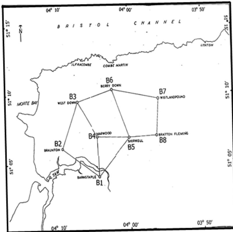
Fig. 12-2 Location map of the base-station network used in the survey. The connecting lines represent the routes along which the base-stations were tied up.
