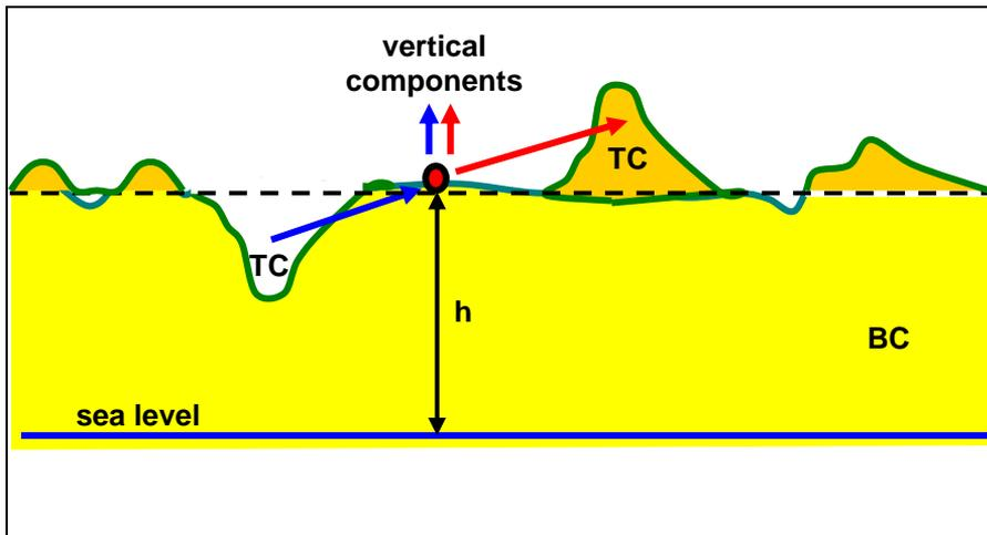
Fig. 7-6 Terrain correction (TC).
