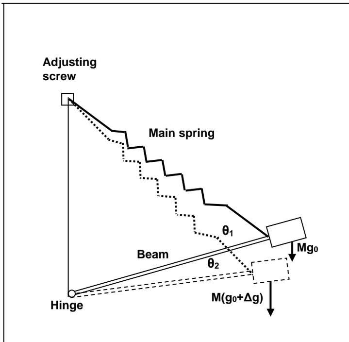
Fig. 5-8 Schematic representation of the LaCoste-Romberg gravimeter.
