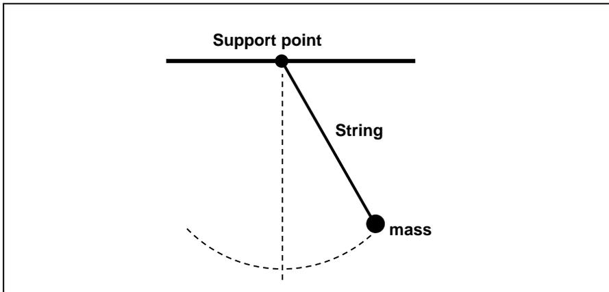
Fig. 5-2 The simple pendulum consisting of a mass attached to the end of a string.
