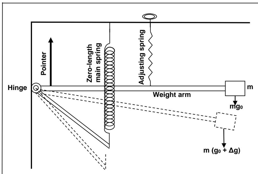
Fig 5-10 Schematic representation of the Worden gravimeter.
