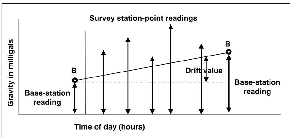
Fig. 6-4 Base station re-occupation during normal survey work
