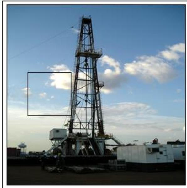
Figure 1.8 A typical rotary drilling rig, set up for oil-well drilling operation.
