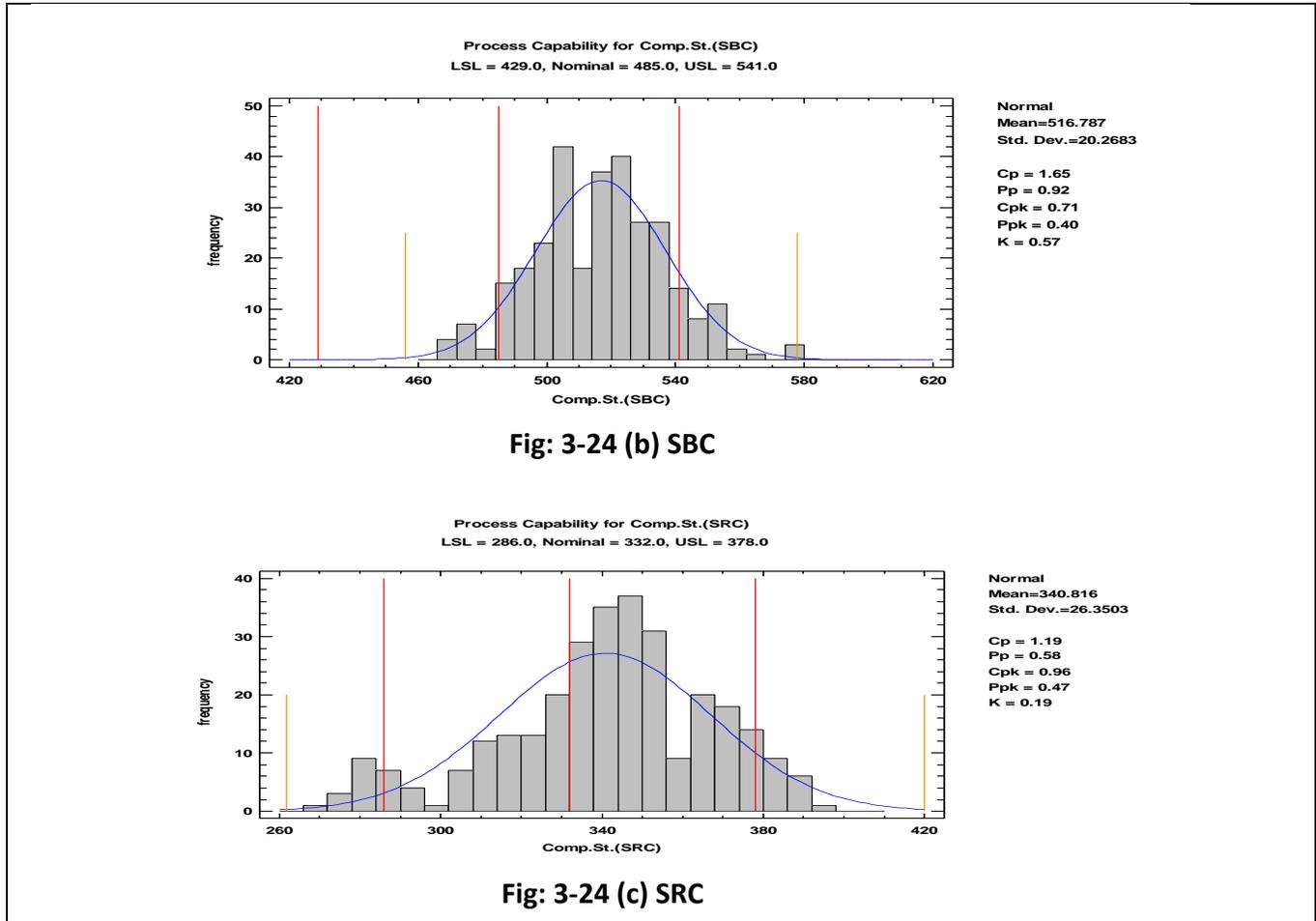
**Figure (3-24): Process capability for Comp.st. (OPC, SBC and SRC)**
