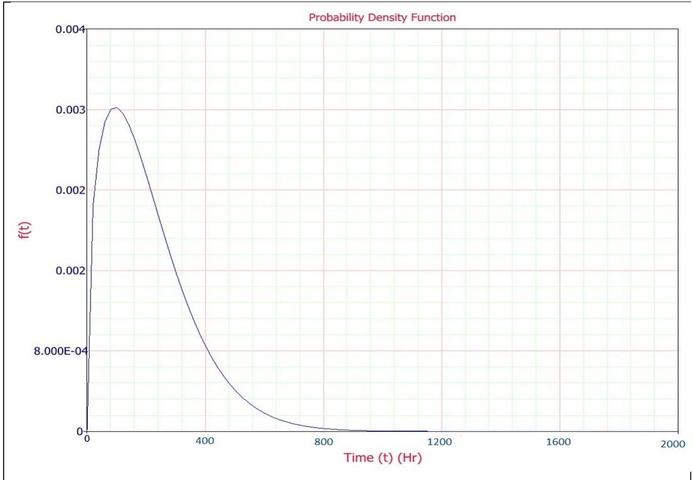
**Figure (3-2): Represents the probability density function of the failure time of cement mill (1)**
