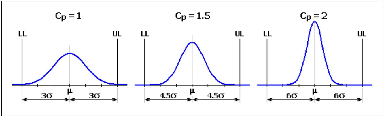
Figure (2- 7): Represents capability index two sides target value = mean
