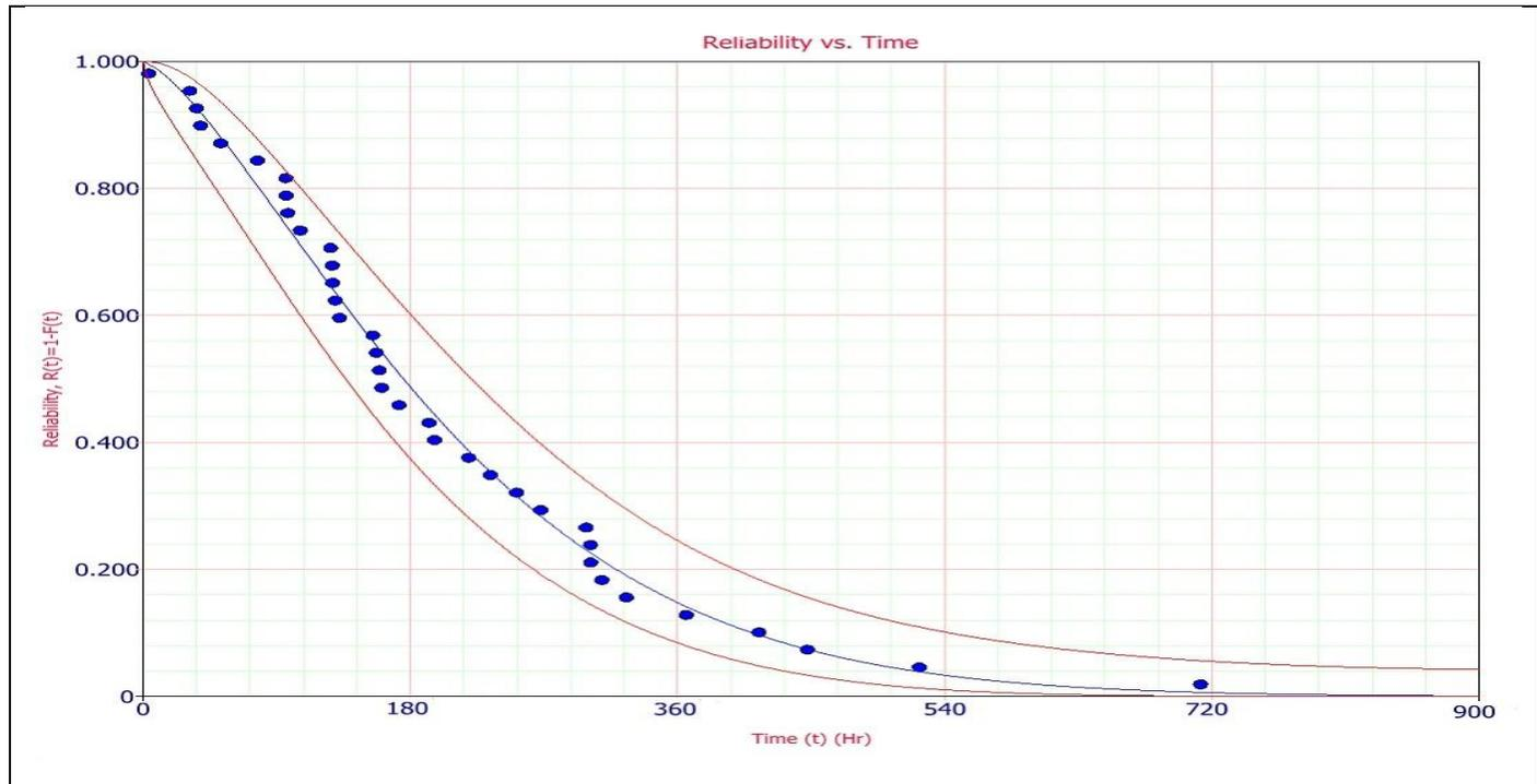
**Figure (3-4):** Represents the reliability of cement mill (1).
