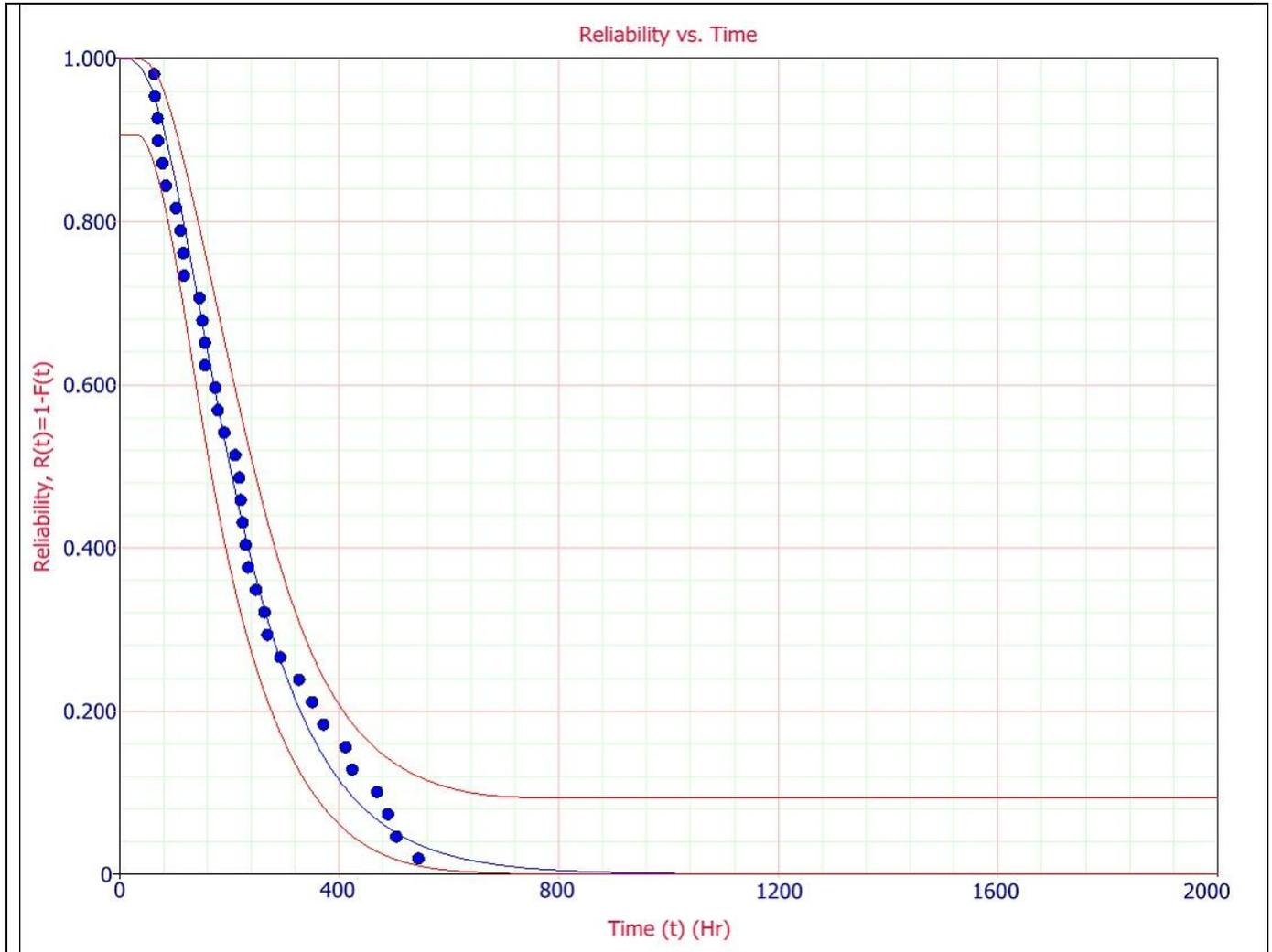
**Figure (3-12):** Represents the reliability of cement mill (3)
