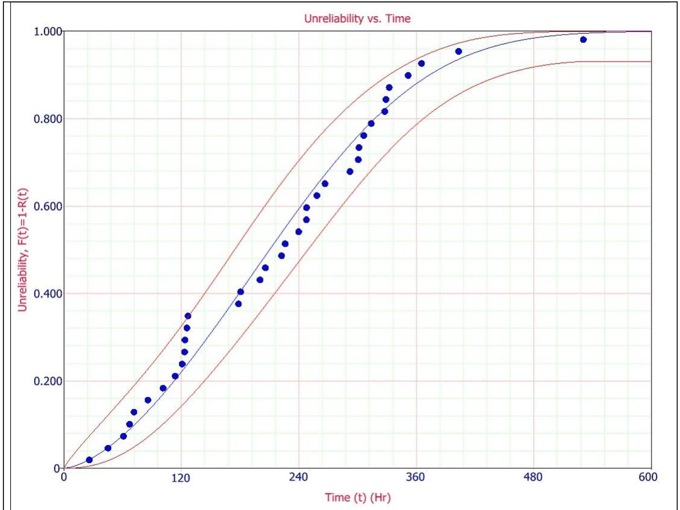
**Figure (3-7): Represents the cumulative distribution function of cement mill (2)**
