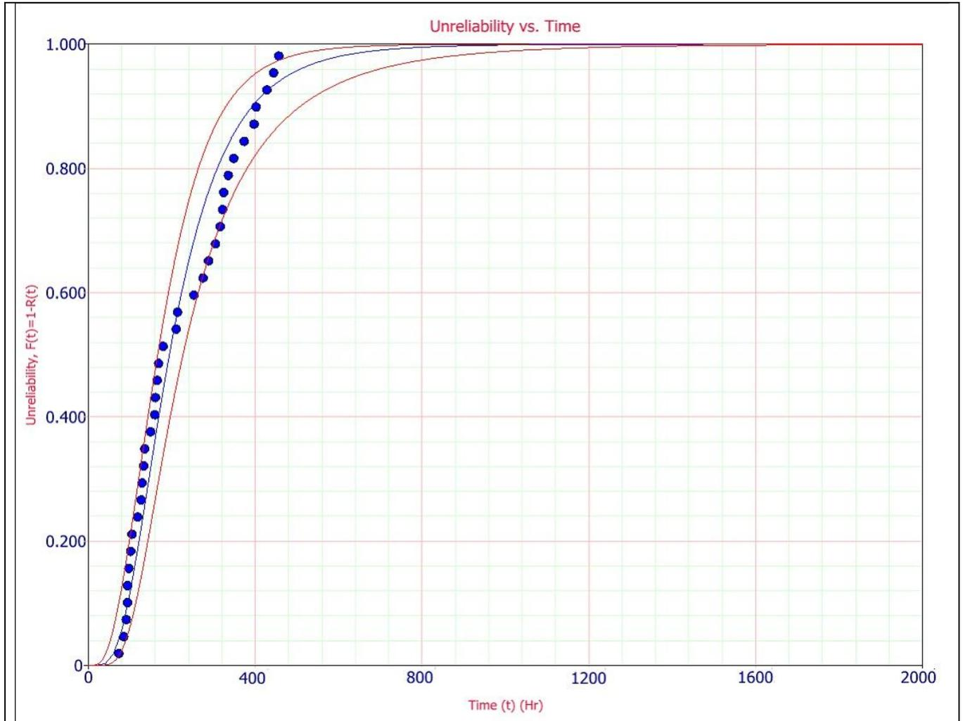
**Figure (3-19): Shows the cumulative distribution function of cement mill (5).**
