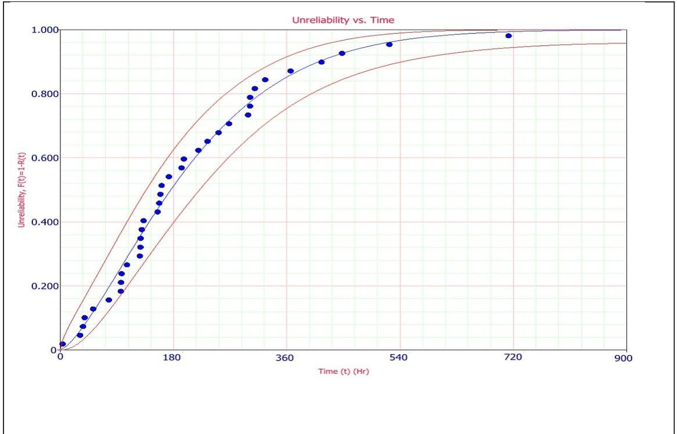
**Figure (3-3):** Represents the cumulative distribution function of failure time for cement mill (1).
