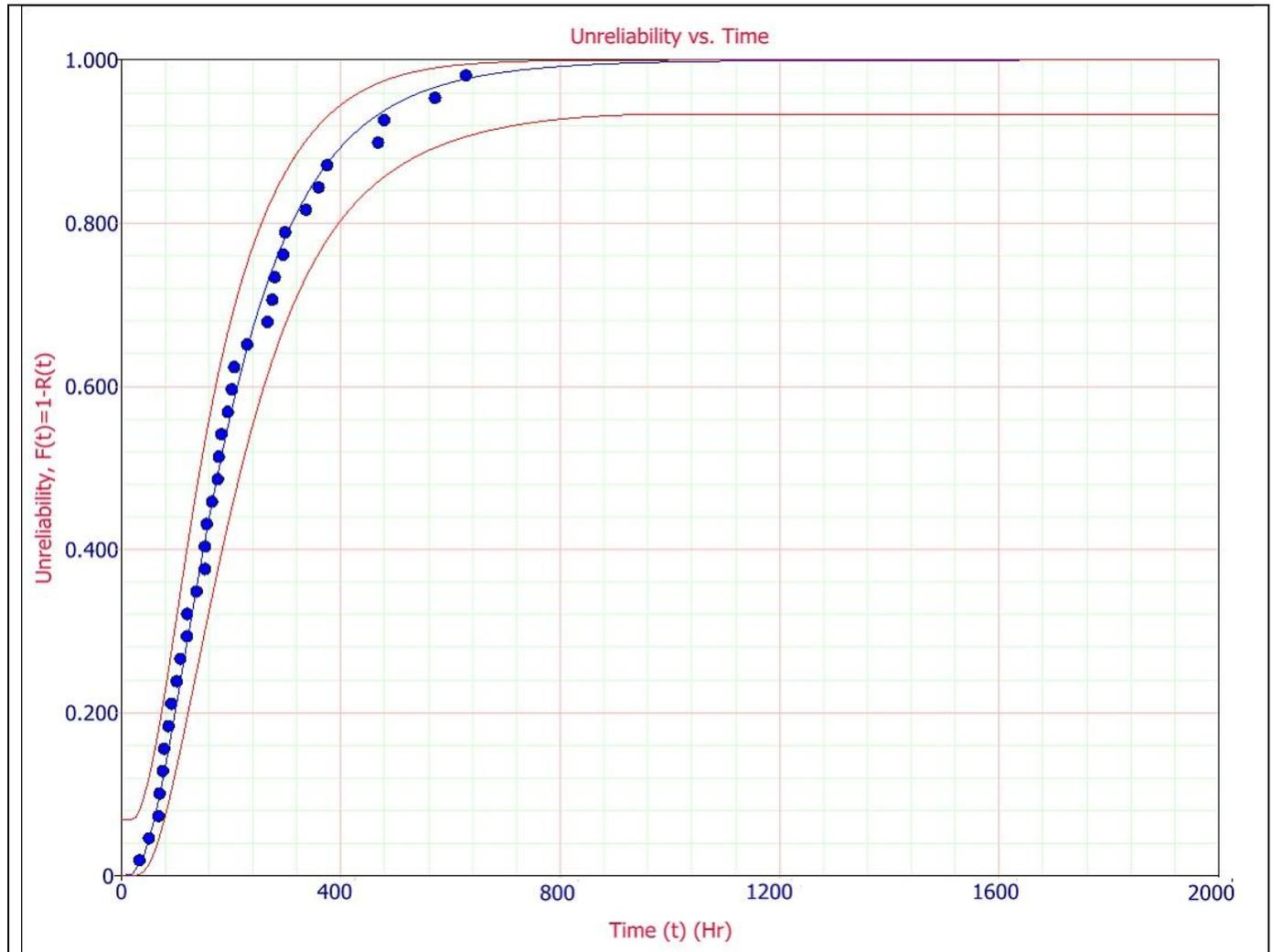
**Figure (3-15): Represents the cumulative distribution function of cement mill (4)**
