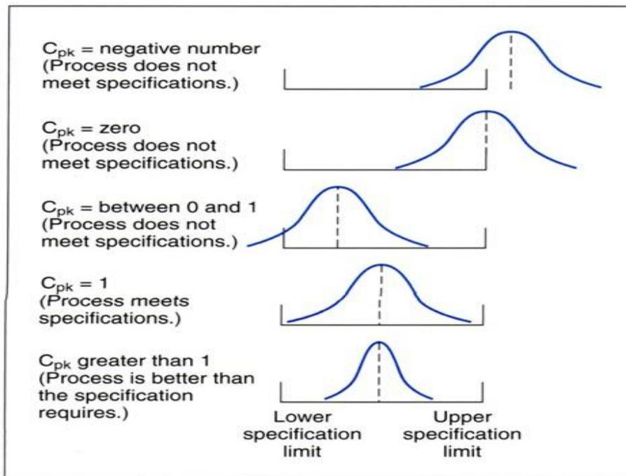
Figure (2- 8): Represents capability index two sides target value  $\neq$  mean
