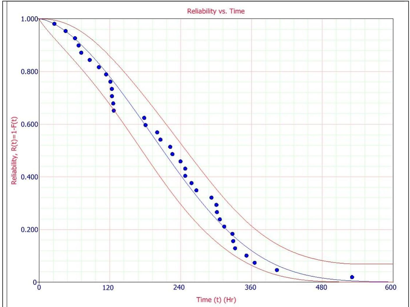
**Figure (3-8): Represents the reliability of cement mill (2)**
