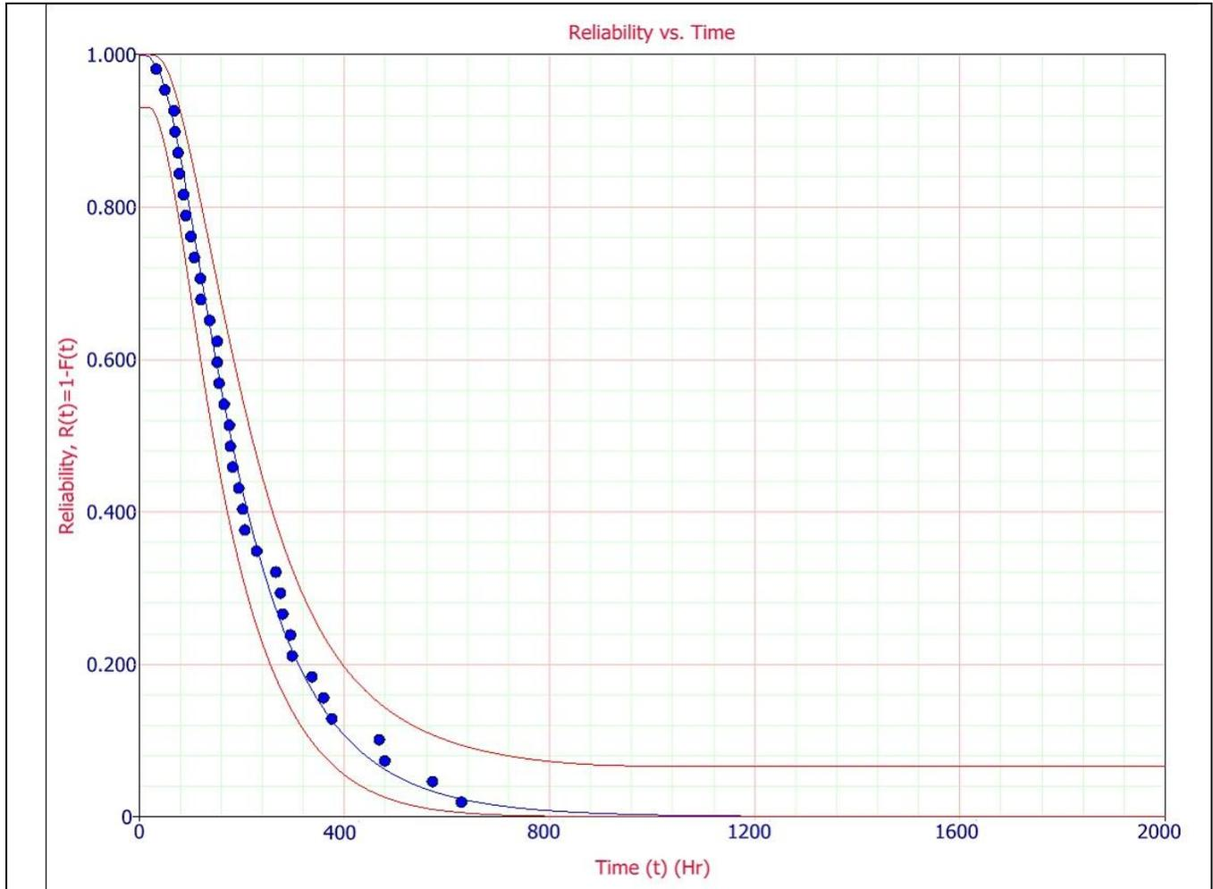
**Figure 3-16: Represents the reliability of cement mill (4).**
