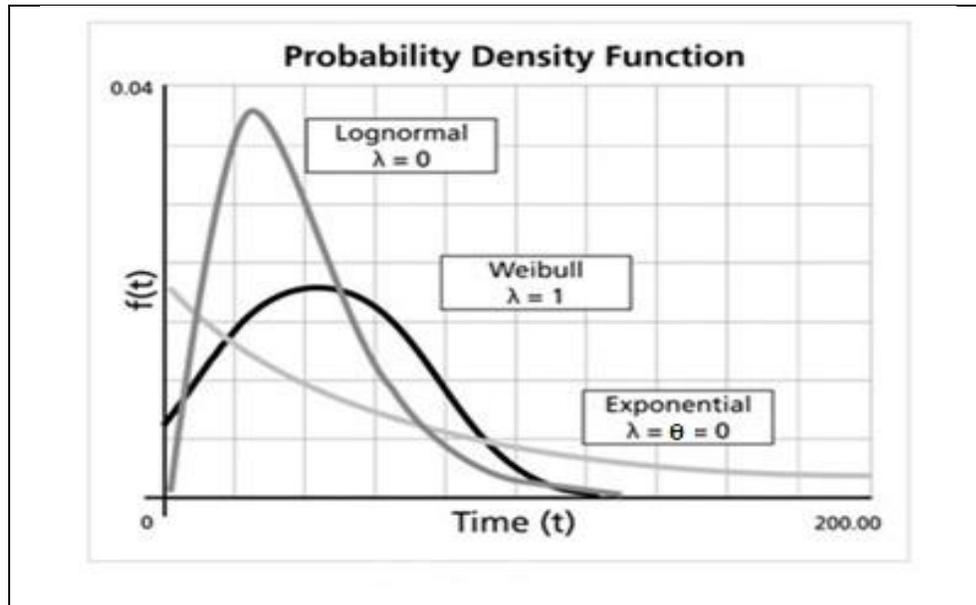
Fig (2-3): Represents the generalized gamma distribution special cases based on the values of the parameters
