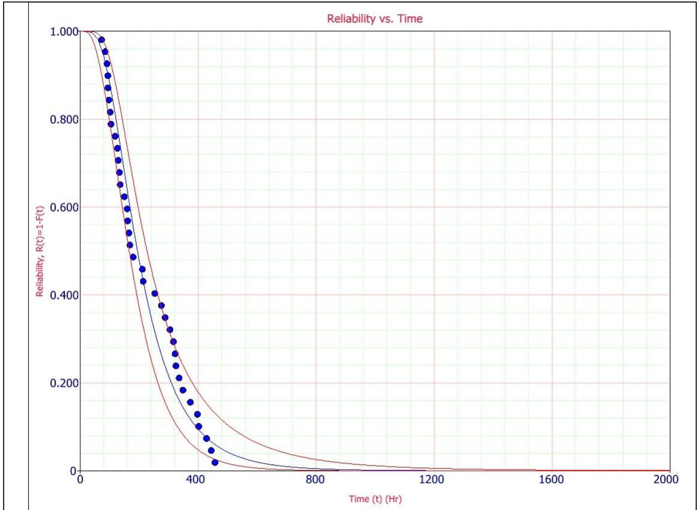
**Figure (3-20):** Represents the reliability of cement mill (5).
