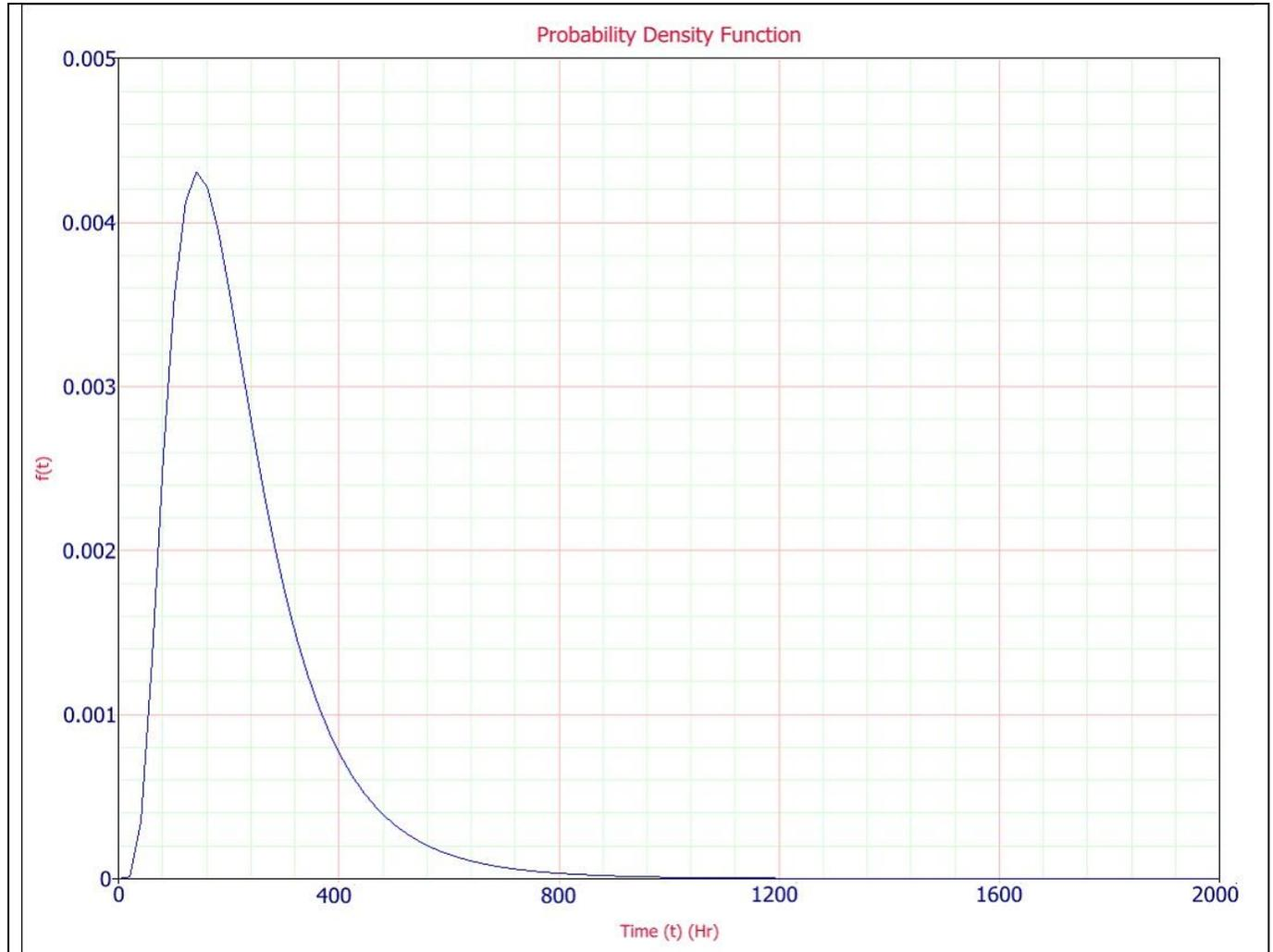
**Figure (3-18):** Represents the probability density function of cement mill (5).
