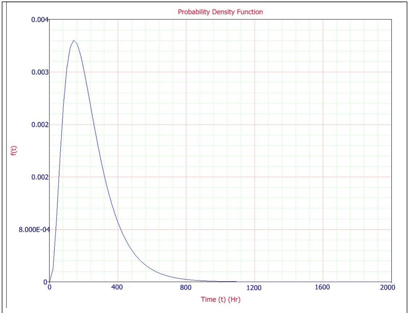
**Figure (3-10):** Represents the probability density function of cement mill (3).
