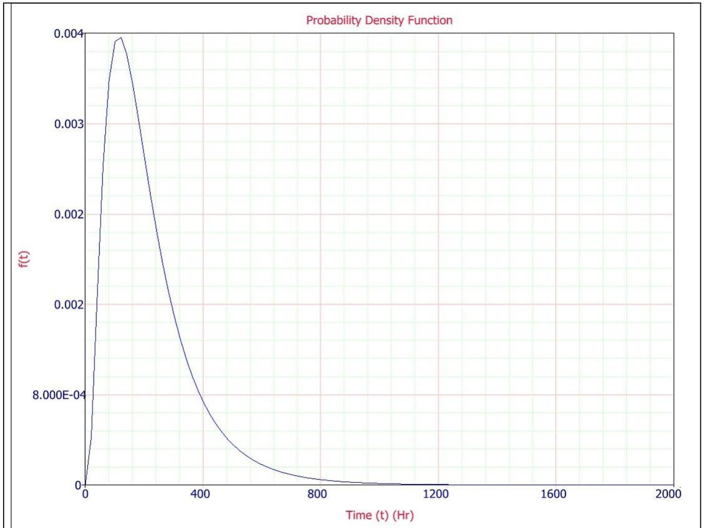
**Figure( 3-14): Shows the probability density function of cement mill (4).**
